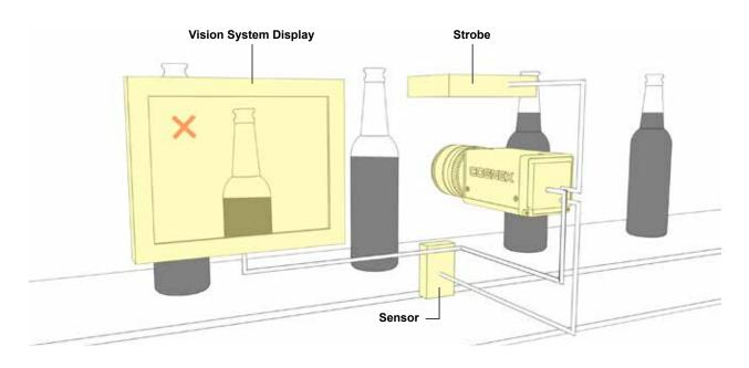
Figure 1. Bottle fill-level inspection example
