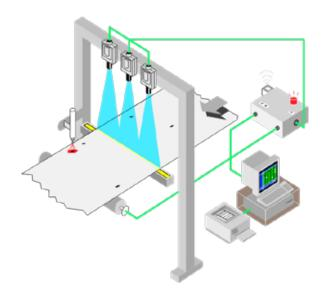
Figure 10. 1D vision systems scan one line at a time while the process moves. In the above example, a defect in the sheet is detected.
