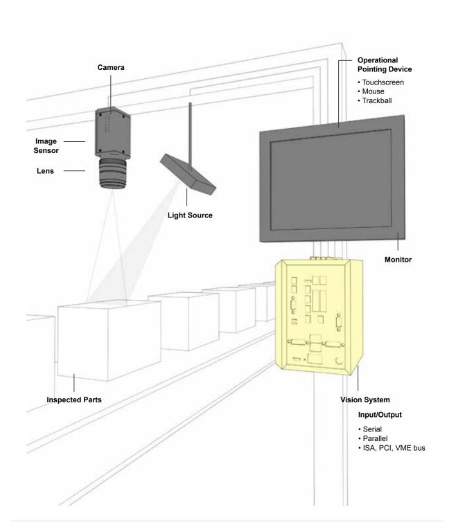
Figure 9. Main components of a machine vision system.
