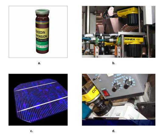
Figure 13. Line scan cameras can (a.) unwrap cylindrical objects for inspection, (b.) add vision to space-constrained environments, (c.) meet high-resolution inspection requirements, and (d.) inspect objects in continuous motion.
