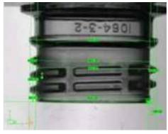
Figure 7. Gauging applications can measure part tolerances to within 0.0254 millimeters.
